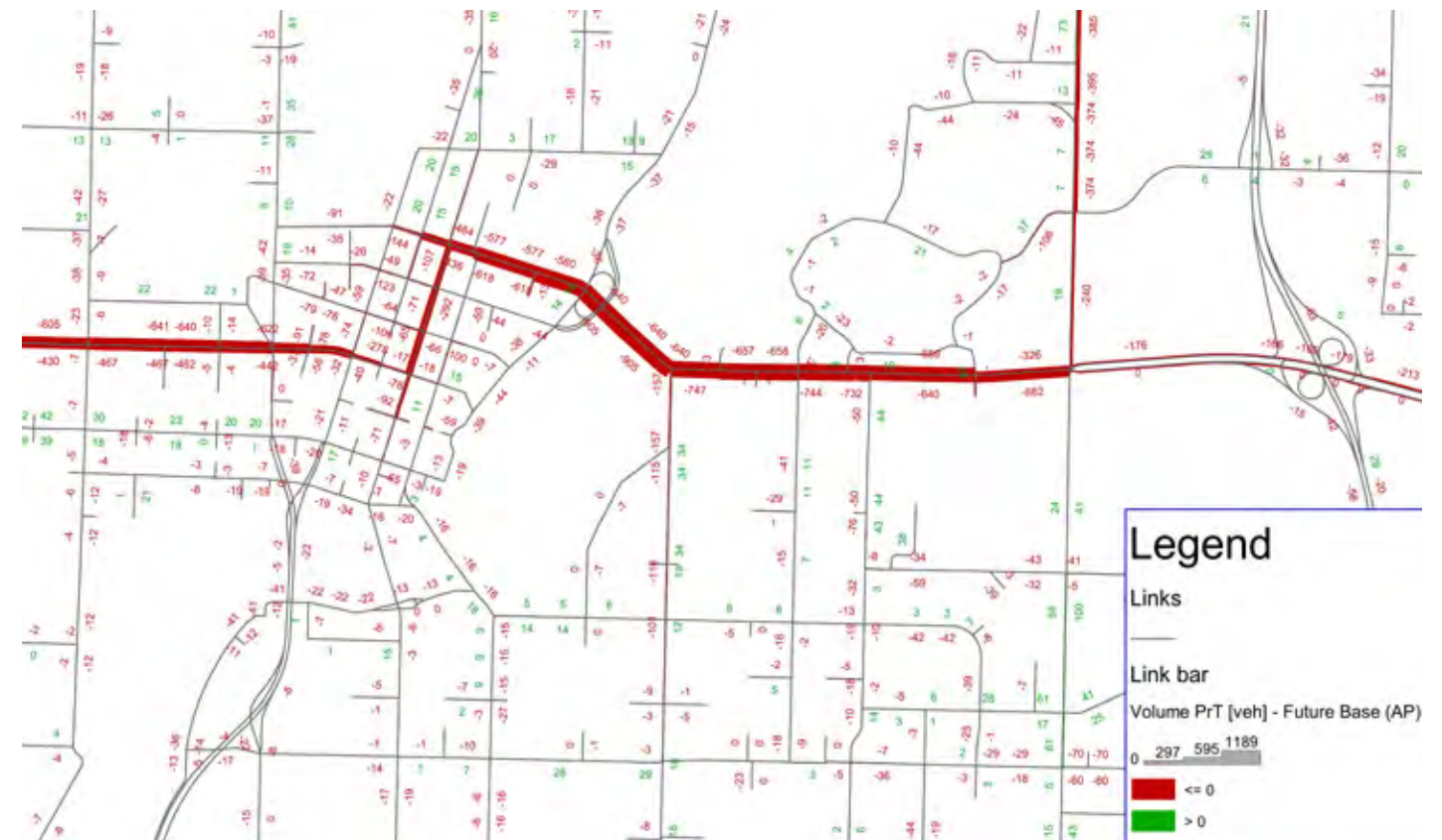
Figure 4.28 - Forecast 2045 PM Peak Hour Traffic Volume Differences (Scenario 2: Future Transit Plan vs. Scenario 1: 'Business-as-Usual')
