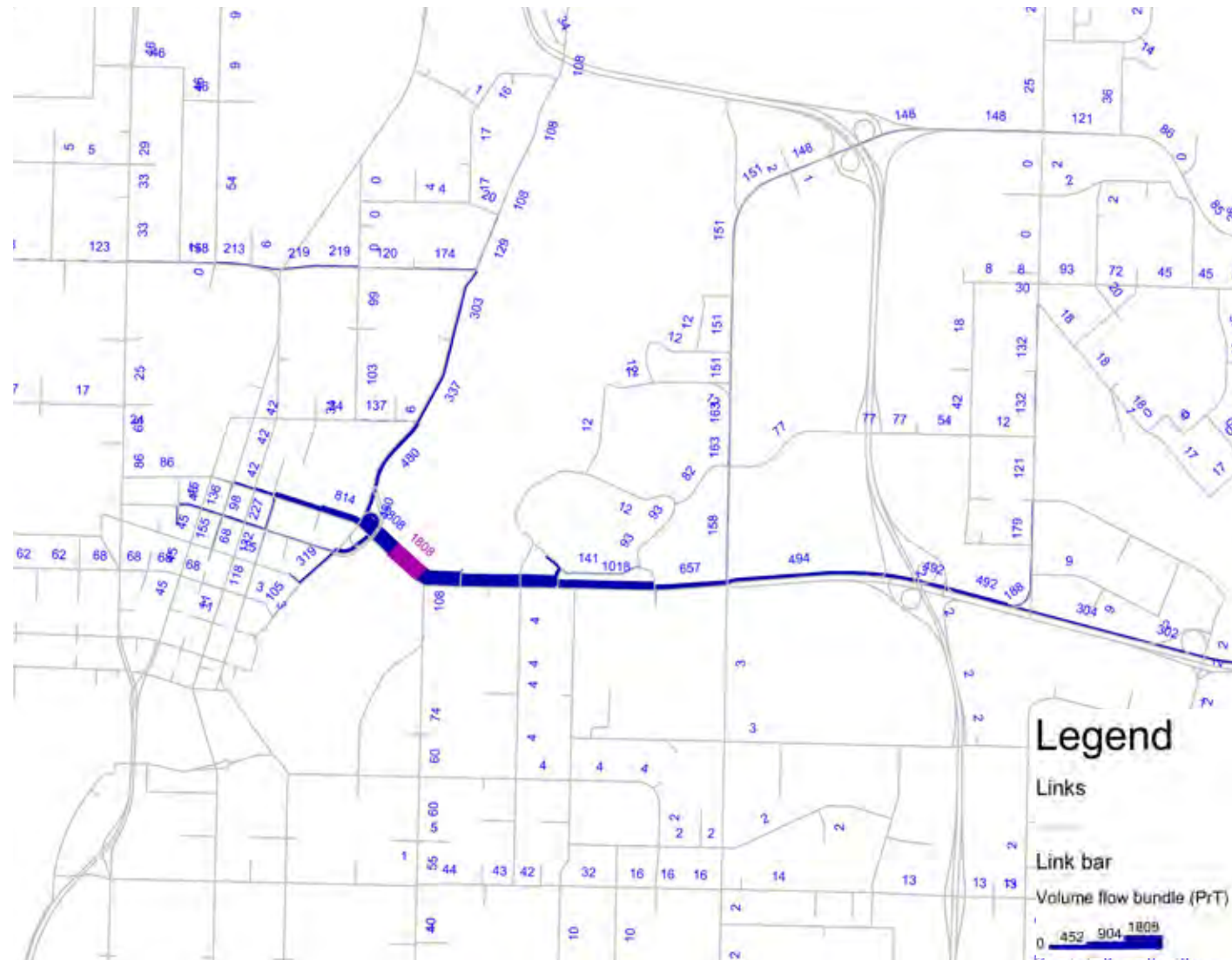
Figure 4.27 - Forecast 2045 PM Peak Hour Westbound Traffic Flow Bundle for University Bridge (Scenario 2: Transit Plan)
