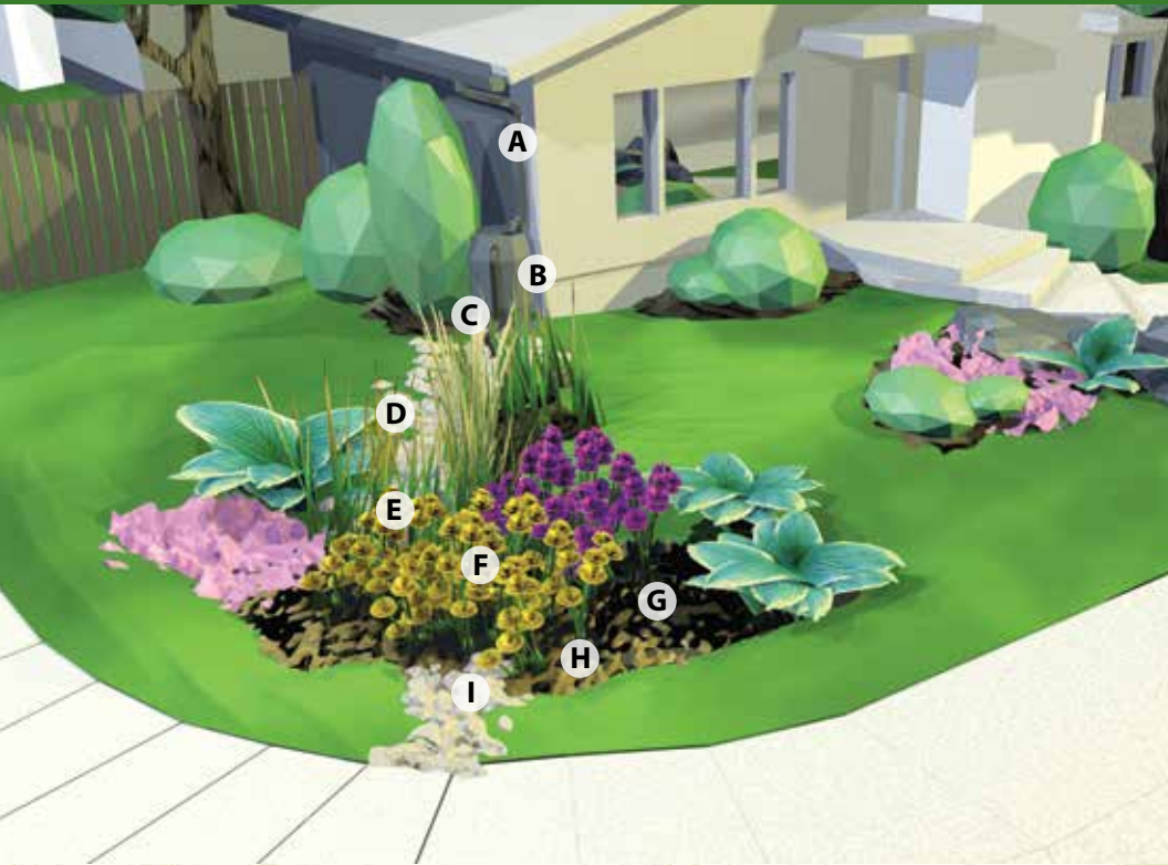
Figure 1: Elements of a Rain Garden
