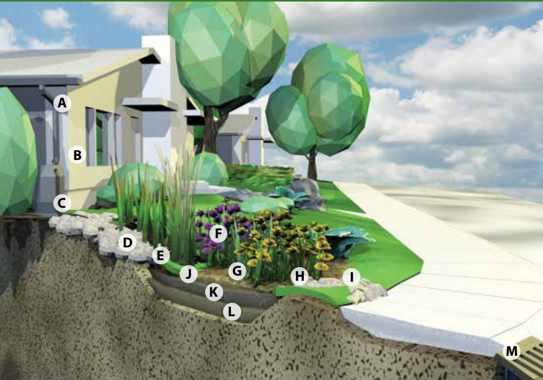
Figure 3: Layers of a Rain Garden
