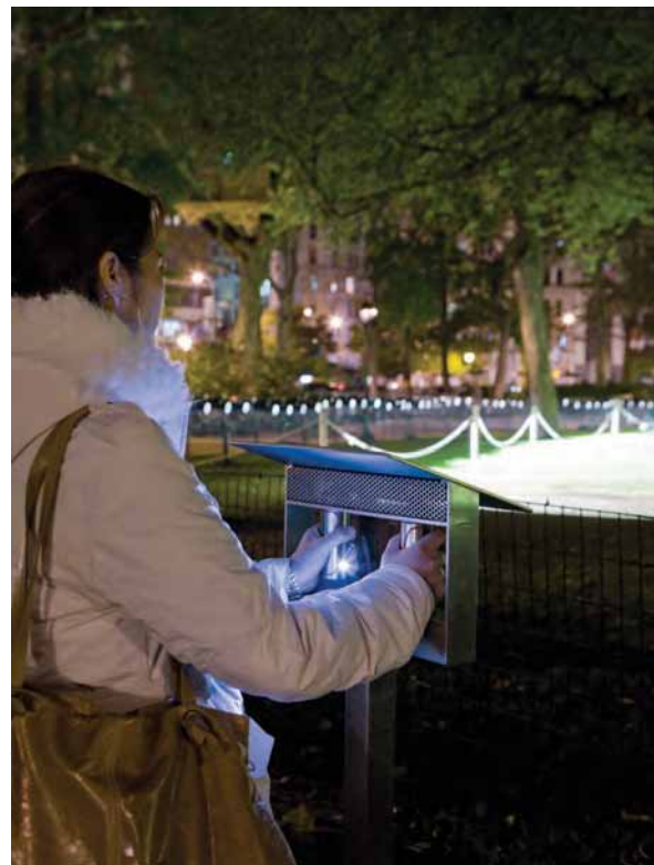
Figure 40 PULSE PARK detail view of the heart rate sensor. (Image Source: Lozano-Hemmer.com).
