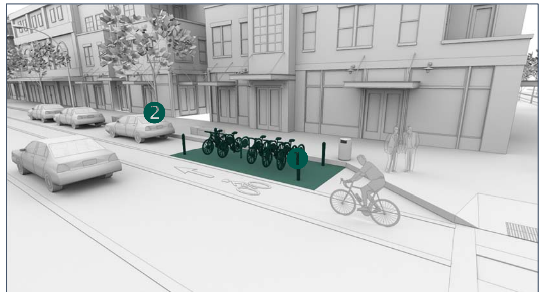
Figure 51 - On-Street Bicycle Parking
