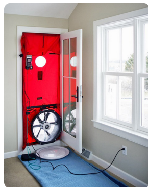
Figure 2: Blower door test
