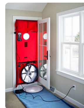
Figure 2: Blower door test
